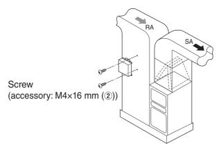
Mount the adapter with the screws (accessory: M4×16 mm (②)) on a place which has sufficient strength and stability.
