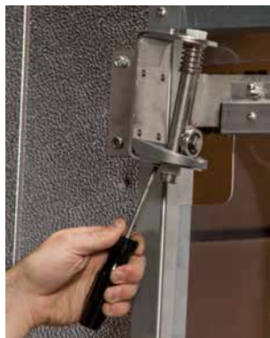
Hinge cam block adjusts with phillips head screwdriver.
