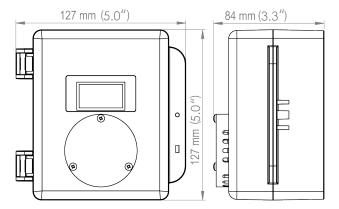
Above dimensions are shown with optional splash guard. Without splash guard, thickness is  $71 \text{ mm} (2.8^{\circ})$ . The area required for enclosure door to be open 90 degrees is  $178 \text{ mm} (7.0^{\circ})$  or  $254 \text{ mm} (10.0^{\circ})$  for fully open. With the optional splash guard installed, the enclosure is IP54 rated.
